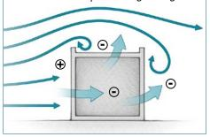
Wind is somewhat predictable, or at least its average speed and direction are. Fans include kitchen and bath exhaust fans, HVAC equipment fans, and clothes dryers. The stack effect generates pressure because warm air rises, pushing up and out on the ceiling in cold weather (see "How It Works" in *FHB* #213 and at FineHomebuilding.com).
