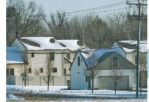
The wind that pushes air into one side of a house also sucks it out the other side. If the outdoor air is moister than the indoor air, water can be driven into framing on windward sides. On a gusty winter day, the pattern of wind pressure can be seen as swirls around corners and edges that sweep snow from specific areas. It is important to have good airbarrier details where roofs, walls, floors, and foundations meet.
